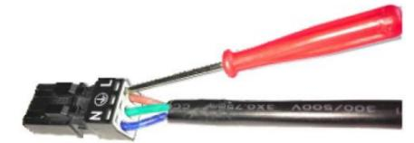
3.3.3 After placing the wires, use the Wire Protection Clip to fasten. Then put on the Shell Base and Shell Cover.
